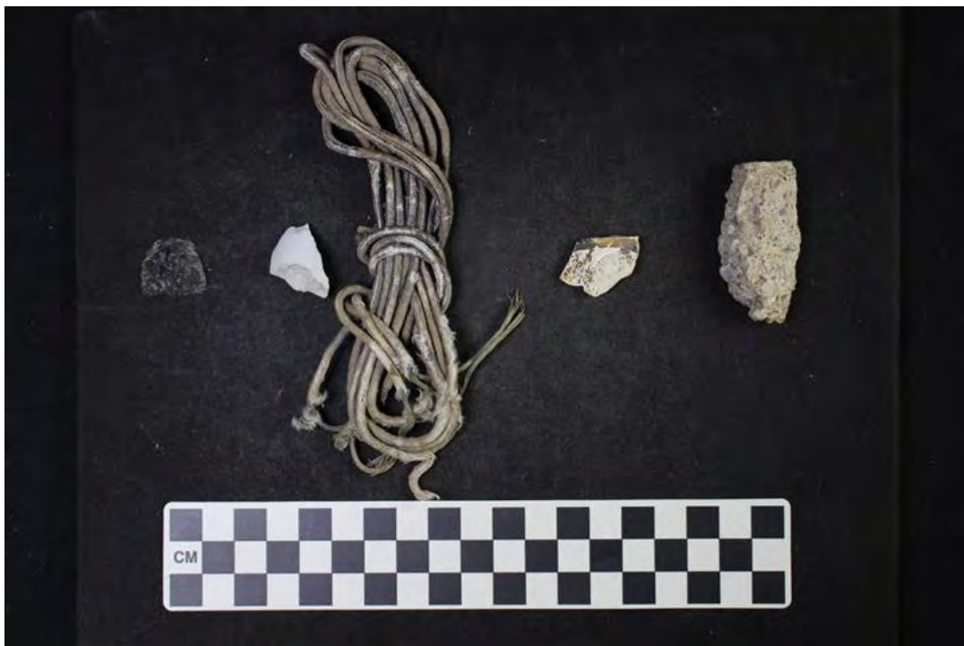
Image 32: Location 4 (AfHh-945); (left to right) asphalt shingle, porcelain electrical insulator, electrical wire, dust-pressed tile, and concrete.
