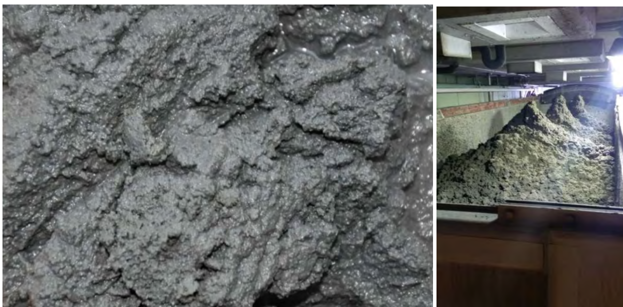
Figure 11 – Water Treatment Plant Process Residuals
