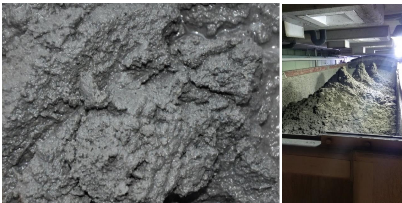
Figure 11 – Water Treatment Plant Process Residuals
